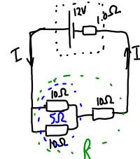
First find the equivalent resistance of the  $3 \times 10\Omega$  resistors:
