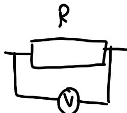
an ideal voltmeter has infinite resistance
