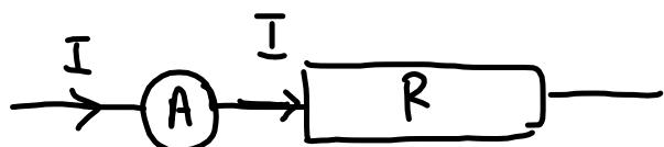
The ammeter must be placed in series and have negligible resistance.
