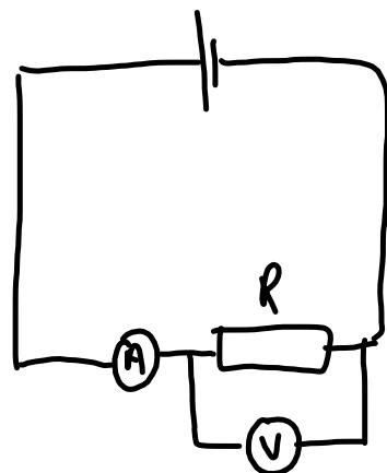
This is suitable if a less than perfect ammeter is used. The pot. diff across it doesn't affect the voltmeter reading.
